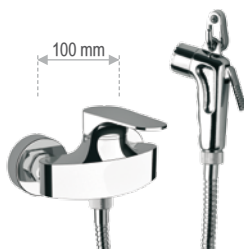
LC 31 DP Miscelatore monocomando esterno doccia, interasse 100 mm, con kit composto da doccetta shut-off in abs cromato art. 332DPCR, flessibile conico in ottone cromato 120 cm e gancio cromato art. 332GA. Wall mounted single-lever shower mixer, interaxis 100 mm, with kit composed by shut-off handshower in c.p. abs art. 332DPCR, conical flexible in c.p. brass cm 120 and c.p. hook art. 332GA.
