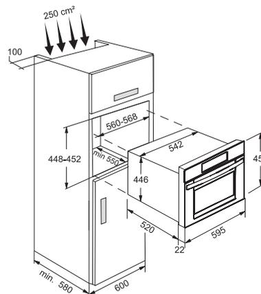
**SCHEMAS D'ENCASTREMENT MACHINE A CAFE**
